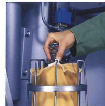
Needs to be cleaned only once a day: the lint filter
