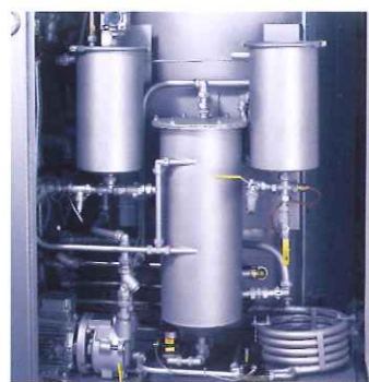
Avoids creation of odour: the multistep water separator
