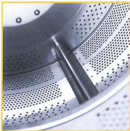
Best possible drying by optimized cage airflow
