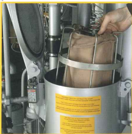
Proven principle: Only one opening for button trap and lint filter on PX models
